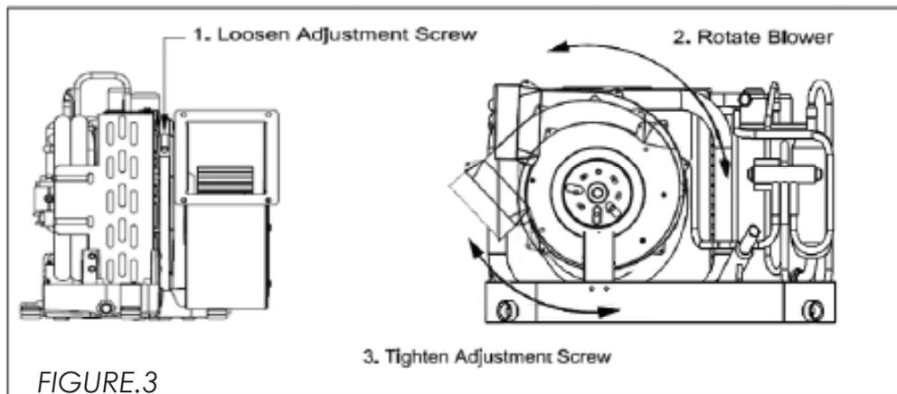
Adjust the air outlet by loosening lock screw and secure the screw tightly once the air outlet is adjusted at the optimal location. See figure 3.
